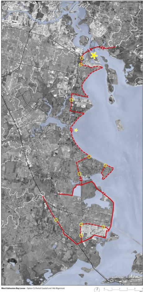
Figure 17. Plan view of the proposed Galveston Bay Shoreline Levee connecting the proposed Centennial Gate with the existing Texas City Levee.
