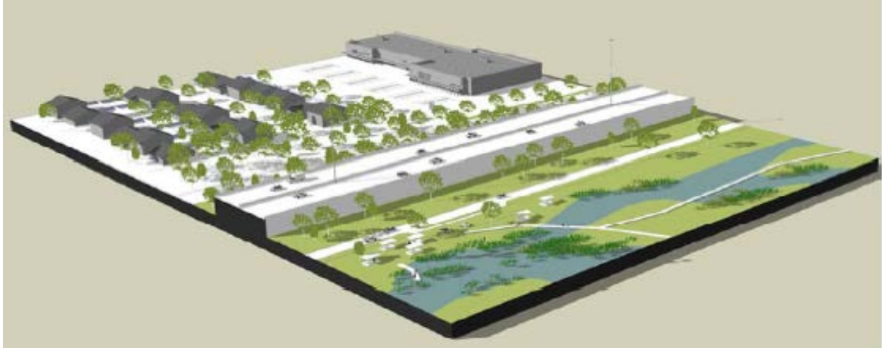
Figure 16. Profile view of the proposed SH 146 Levee after buy-out of east side of SH 146.
