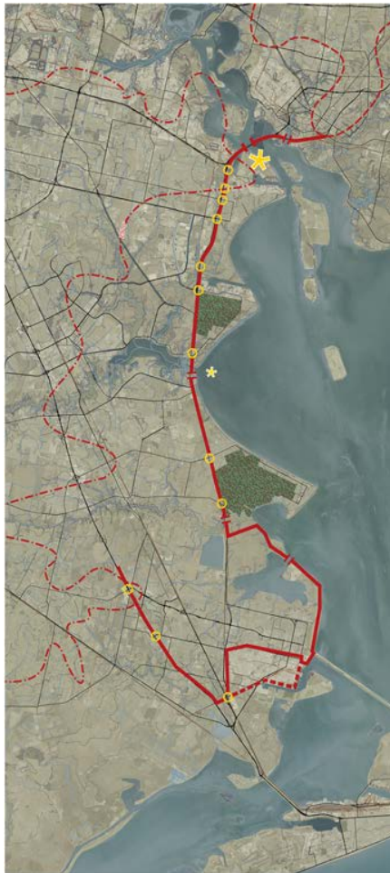
Figure 15. Plan view of the proposed SH 146 Levee connecting the proposed Centennial Gate with the existing Texas City Levee.
