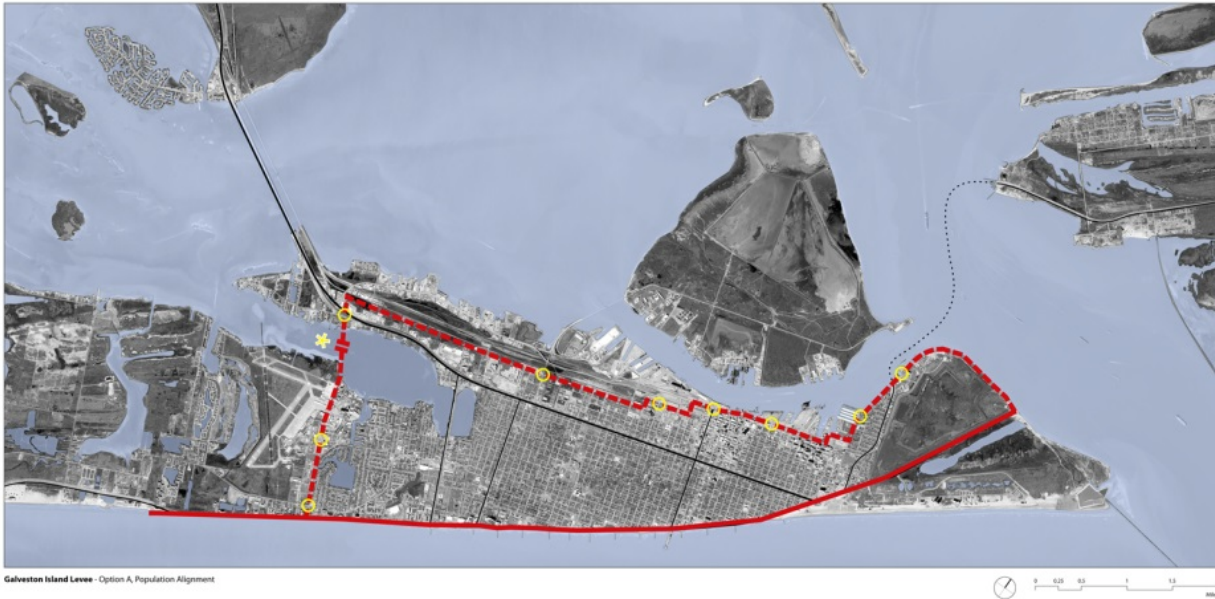
Figure 20. Proposed backside levee extending from the Seawall along Harborside, crossing Offatts Bayou and connecting back to the seawall east of the airport.
